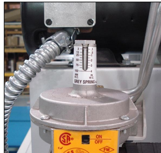
Figure 11. Airflow interlocking safety switch.
